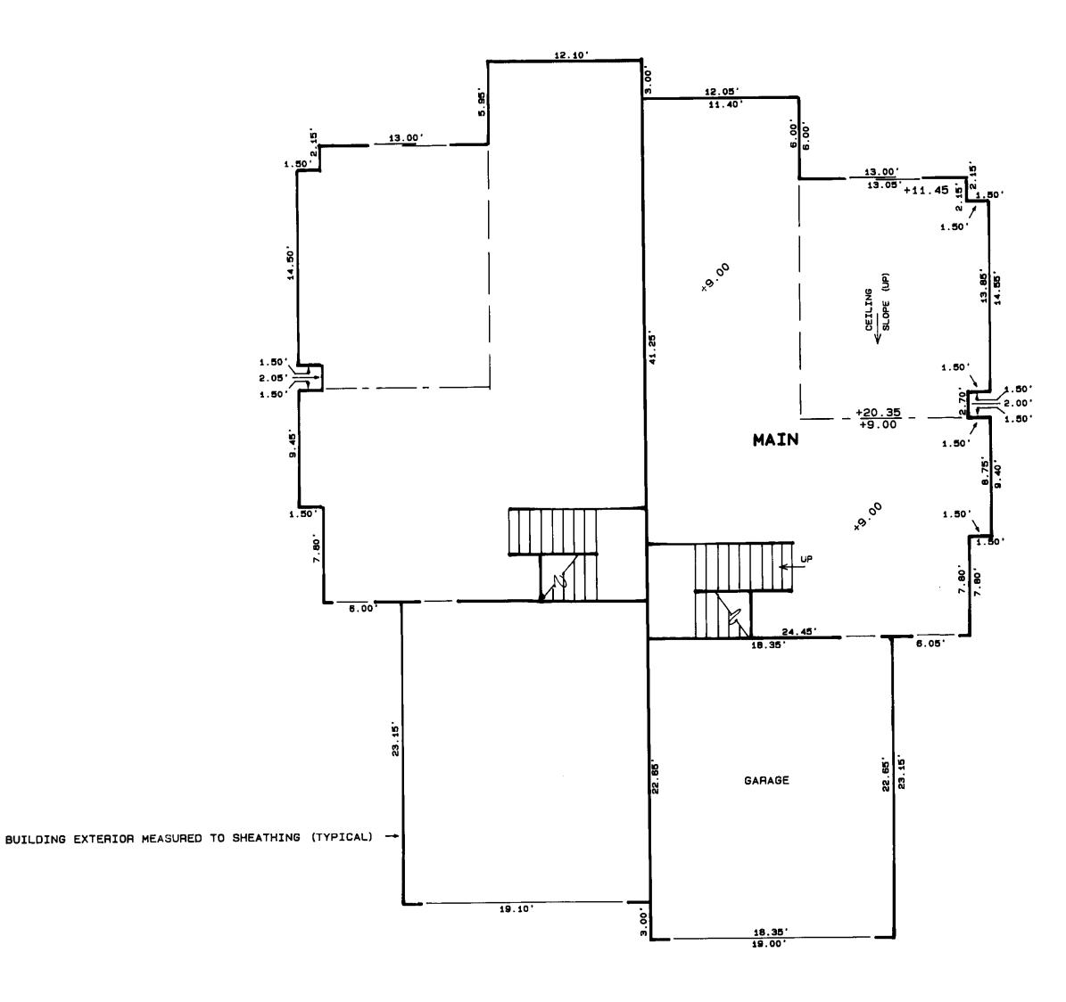
BUILDING EXTERIOR DIMENSIONS FOR UNITS 3 / 4, 5 / 6 AND 7 / 8 FLOOR PLAN FOR UNIT TYPE 'B' (NO SCALE)
