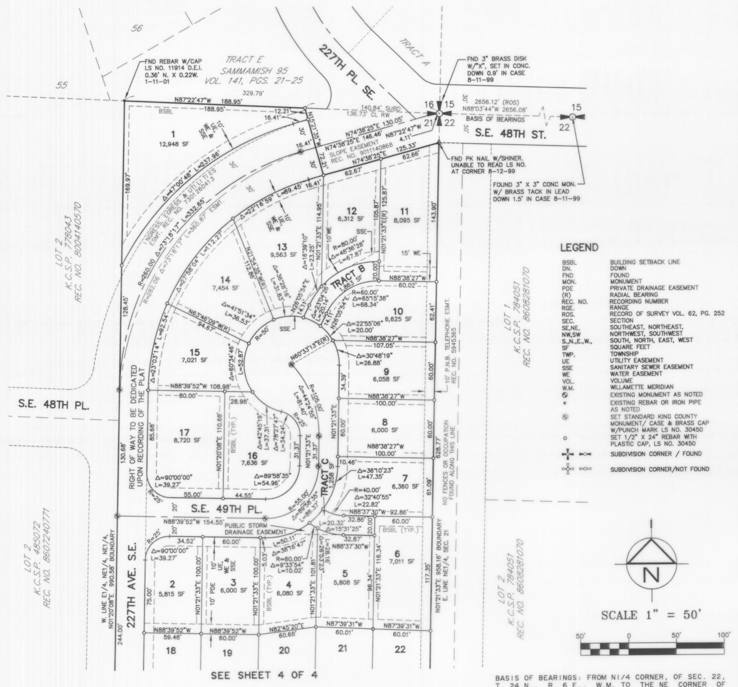
BASIS OF BEARINGS: FROM NI/4 CORNER, OF SEC. 22, T. 24 N., R. 6 E., W.M. TO THE NE CORNER OF NE CORNER OF SEC. 21, PER RECORD OF SURVEY RECORDED IN VOLUME 62 OF SURVEYS, PAGE 252, = N88°03'44"W.
